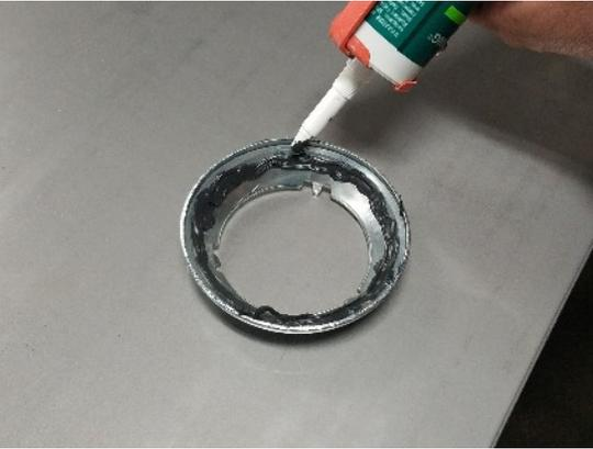
Step 1: Add a bead of adhesive to the inside of the Neckring skirt/Neckring sleeve.
