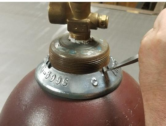
Step 3: Peen over the three locking tabs into the threads of the existing neckring.
